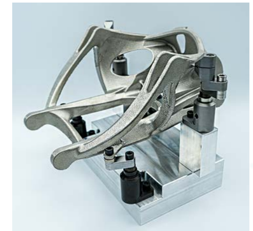
Clamped part ready for CNC machining
